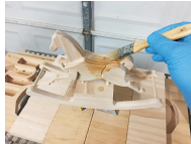
Applied thinned Seal Coat
