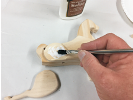
Glue the legs to the body assembly
