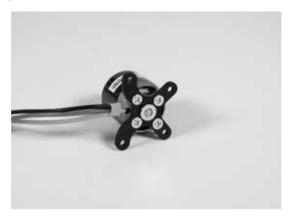
2. Attach the Outrunner motor to the front of the firewall using four 4-40 x 1 <sup>1</sup>/<sub>4</sub>" socket head screws and the aluminum motor spacers.
