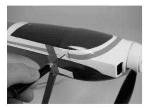
O 6. Enlarge the holes in the cowl using a 5/64" (2mm) drill bit. Secure the cowl using four 2mm x 8mm sheet metal screws. Snap the spinner cone onto the spinner backplate once the cowl is secure.
