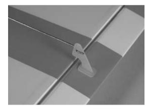
○ 4. Plug the aileron servo into the receiver. Power up the transmitter and receiver. Center the aileron stick, trim, and any programmed sub-trim values. Install the arm on the servo so it is parallel to the aileron hinge line. Use a 2mm x 4mm screw to secure the linkage.
