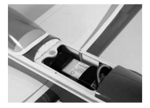
**Note**: Place a piece of hook and loop tape on the bottom of the battery and on the fuselage where the battery rests. This will keep the battery from shifting forward or backward during extreme maneuvers. 7. Install the battery hatch to the top of the fuselage. The magnet will hold the battery hatch in place.
