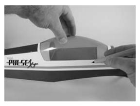
○ 3. Use medium grit sandpaper to roughen the covering 1/8" (3mm) inside the line drawn. Also roughen the outside 1/8" (3mm) of the canopy. Clean the sanded areas using a paper towel and rubbing alcohol.
