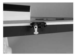
O 6. Remove the servo arm from the elevator servo. Drill a 1/16" (1.5mm) hole through the center hole in the arm. Slide the control connector through the hole and secure it using the connector backplate.
