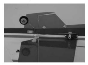
O 9. Repeat Step 7 for the rudder linkage.
