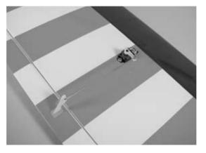
O 5. Repeat Steps 1 through 4 for the remaining aileron servo. Then connect a 6" Y-harness to the two 6" servo extensions on the servos.
