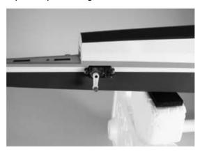
○ 8. Locate the 4" (102mm) linkage wire. Slide the "Z" bend into the center hole of the elevator control horn. Pass the linkage through the pushrod connector on the servo arm. Turn on the radio and plug the elevator servo into the receiver. Center the elevator trim and stick, and check that the sub-trim (if a programmable radio) has been set to 0. Install the servo horn back onto the elevator servo. Use a 2mm x 4mm screw to secure the linkage.
