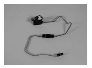
○ 5. Install the elevator servo into the fuselage using the hardware provided with the servo. Drill 1/16" (1.5mm) holes into the fuselage for the screws.
