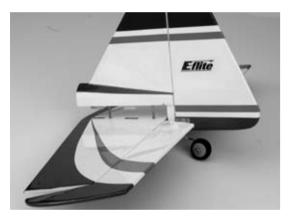
3. Slide the rudder/stabilizer assembly onto the fuselage. Slide the #4 washers onto the threaded rods. Thread the nuts onto the rod, tightening them snugly against the bottom of the fuselage.
