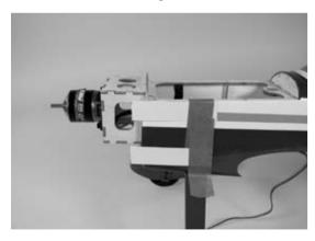
4. Slide the cowling onto the fuselage. Install the propeller adapter onto the Outrunner shaft. You may need to ream out the hole on your prop hub to fit the prop adapter shaft at this point. Slide the propeller onto the prop adapter shaft. The spinner backplate and spacers may need to be enlarged as well to fit the prop adapter. Slide the spinner backplate and any needed spacers onto the prop adapter shaft. Secure the propeller using the prop adapter spinner and be sure it is secure and tight.
