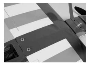
O 6. With the aircraft fully assembled, install the battery into the battery compartment. Secure the battery using the hook and loop tape and a hook and loop strap.
