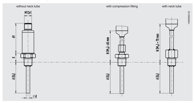
1) At a process temperature of > 150 °C [302 °F], a neck length N (MH) of 70 mm is necessary, otherwise N (M<sub>H</sub>) selectable (55, 65 or 70 mm).
