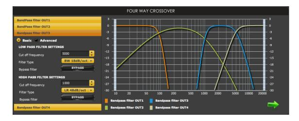
In the miniDSP 2x4 plugins, each output channel has a high pass filter and a low pass filter, each of which can be set to one of a range of filter types and slopes, or individually bypassed. Clicking on the bars labeled "CH1 Bandpass Filter OUT1," and so on displays the filter parameters for that output channel.
