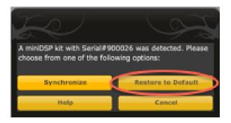
Click on the **Restore to Default** button. This is essential the *first time you connect to the miniDSP*, as it ensures that the miniDSP hardware unit contains an internal set of data that it understands. (Subsequently, you will generally use the **Synchronize** button.)
