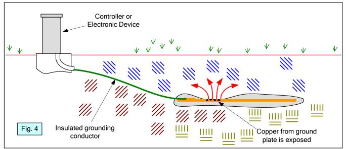
**The generic solution** - Figure 5 shows a copper ground plate that is connected to the irrigation controller with an insulated copper grounding conductor. All the bare copper (and some of the insulation of the grounding conductor) is completely surrounded by a soil amendment. Since all the bare metal is in contact with exactly the same type of soil (amendment), the probability of creating a corrosion cell is virtually eliminated.
