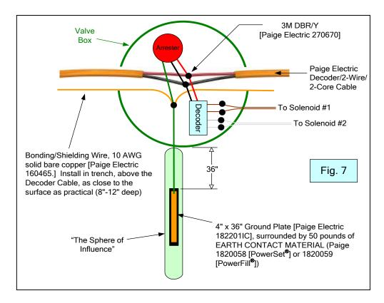
Figure 7 is for a decoder/receiver that uses external lightning arresters.
