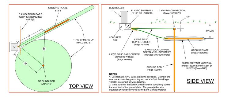
**Grounding Decoder** ٠ systems – Figures 6 & 7 show the proper methods for grounding decoders and other electronic equipment in Decoder/2-Wire/2-Core systems. Also shown are details on how to bond ground grids to each other. The bonding wires are then used for shielding the Decoder/2-Wires/2-Core cables from lightning surges. Figure 6 is for a decoder with an integral lightning arrester and that incorporates a ground wire.
