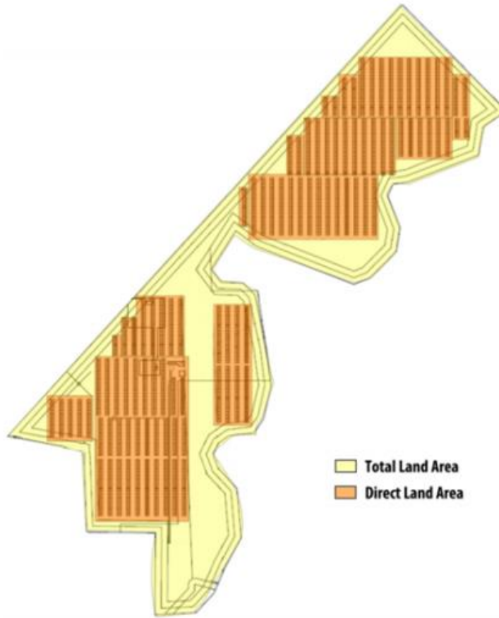
Figure 19: NREL mesa top PV system - example of direct and total land use [64]
