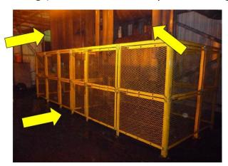
Two conveyor gravity take-up counterweight guarding (source: Belt Conveyor Guarding)
