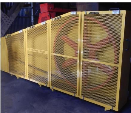
Example of guarding the flywheel of a crusher. (source: Belt Conveyor Guarding).
