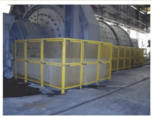
Example guarding in the vicinity of a grinding mill (source: Belt Conveyor Guarding).
