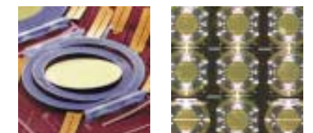
Left: Micro electronic mirrors Right: Switch element
