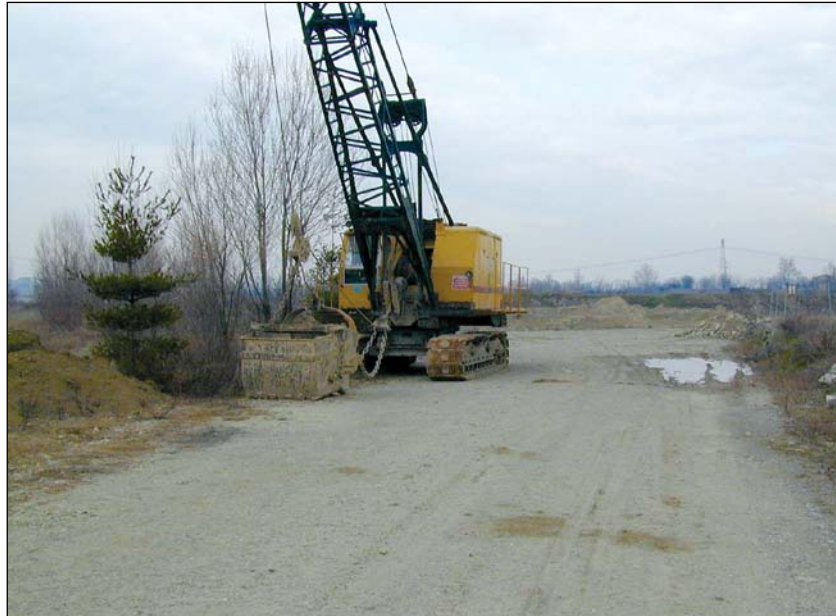
Figure 3.15: Draglines can be used to excavate sand and gravel from a stream channel (Langer, 2003)
