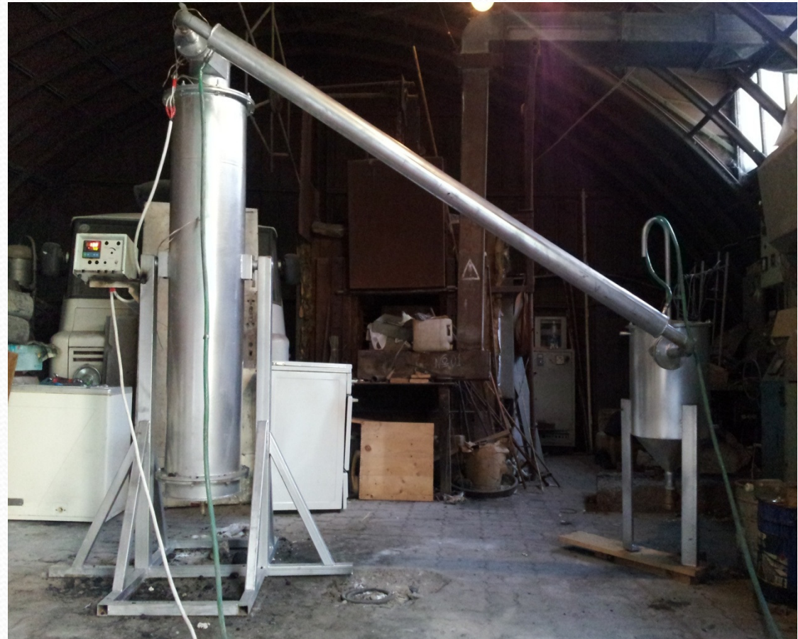
Figure 8. Pilot installation for thermal processing of oil sands
