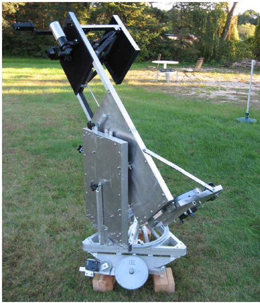
10" flatscope Newtonian mounted on the equatorial platform, viewed from the north.
