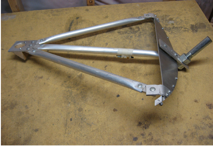
The upper (moving) part of the platform.
