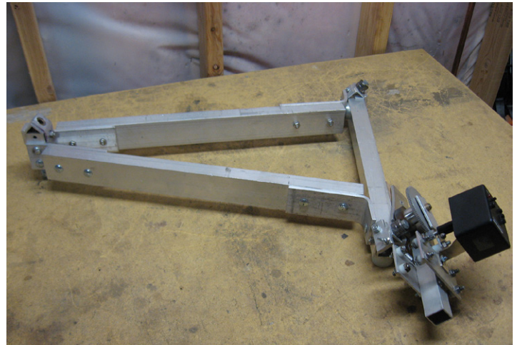
The base of the platform with the upper part removed.
