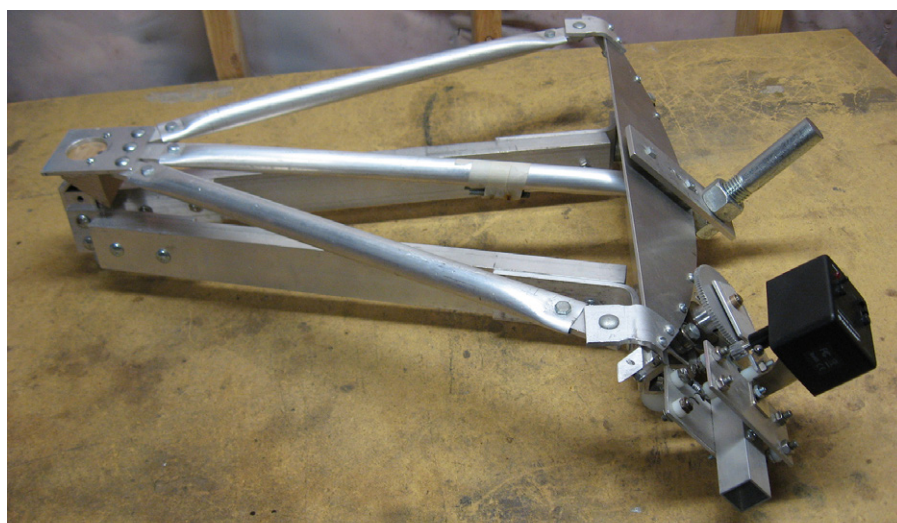
Side view of the equatorial platform. South pivot is at the left. At the right are the north arc, drive mechanism, and bar for counterweights.
