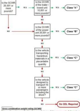
Means the value specified by the manufacturer of the power unit, if the value is displayed on the Federal Motor Vehicle Safety Standard [FMVS5] certification label; or the sum of the gross vehicle weight ratings (GVWRs) or the gross vehicle weights (GVWRs) of the power unit and the towed unit(s), or any combination thereof, that produces the highest value.
