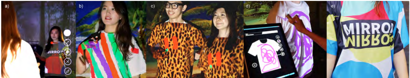
Figure 1. Mirror Mirror is a design system that combines Spatial Augmented Reality with a mirror display. Virtual garments are visible in the mirror reflection (a) as well as on the body (b). Multi user interaction is supported (c, d) and designs are readily printed (e).
