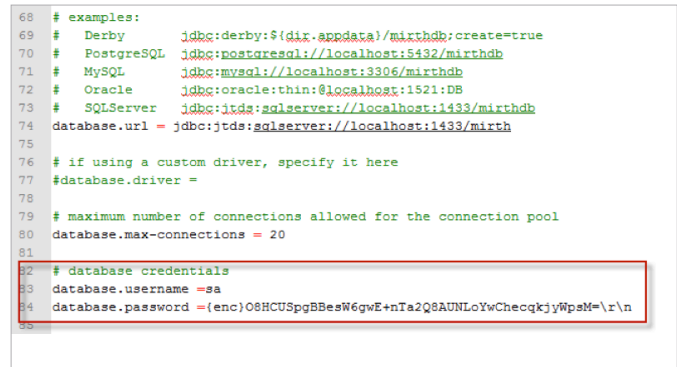
Figure 1.3: Mirth.properties file after encryption settings have been set. The database.password property is now properly encrypted.
