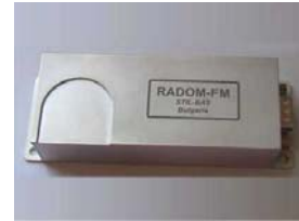
RADOM : characterise the radiation environment in near lunar space.
