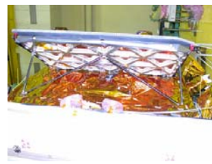
Mini-SAR : Radar system can operate as an altimeter / scatterometer, radiometer, and as a synthetic aperture radar imager.
