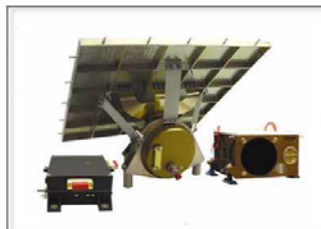
SIR2 : NIR point spectrometer for determination of the chemical composition of crust and mantle
