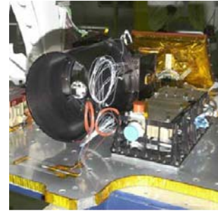
LLRI : Laser altimeter with altitude resolution of < 10m. Slope information in addition to range information.
