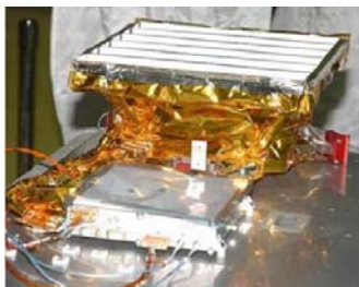
M3 : Imaging spectrometer, operating upto \mu\text{m} range for measuring solar reflected energy.
