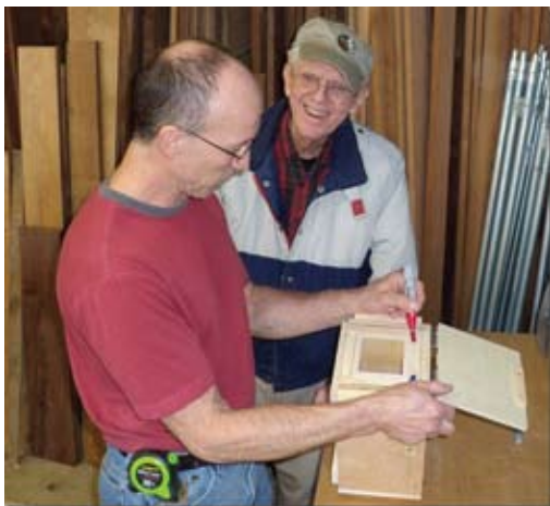
Rodney Montgomery designed a jig for the nestbox to ensure that all of the boxes would be made precisely the same.
