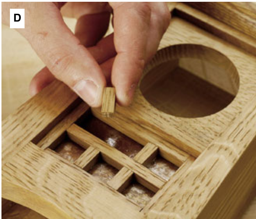
D Install the remaining grille rail and uprights in position, pressing the epoxied edges against the mica. Check for proper alignment.
