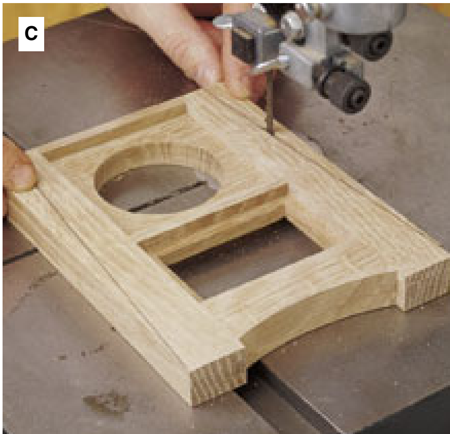
C Bandsaw the stiles to the marked lines to form the tapered sides. Start the cut at the bottom of the stile, and finish at the top. Sand smooth.
