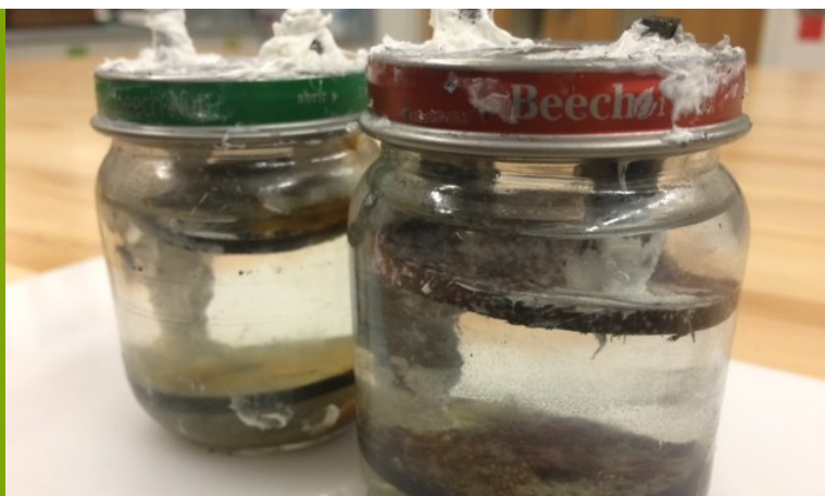
The Zinc Bromide battery cells that Team 2 is using as their power mechanism.
