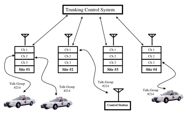
In this illustration shows three cars and one control station radio on the same talk-group. The control system has assigned radio channels at three different sites in order to establish the call. The two cars on the left are both registered on the same radio site while the other units are registered on different sites.
