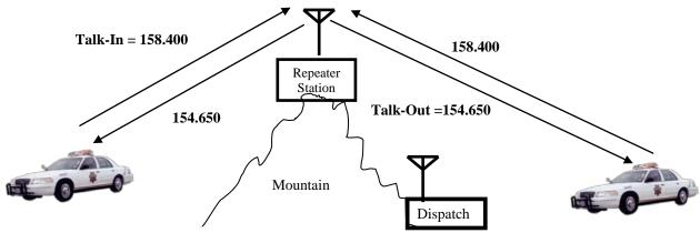
As illustrated above, the repeater receives the frequency being transmitted by the patrol cars (talk-in or repeater input) and the patrol cars receive the frequency being transmitted by the repeater (talk-out or repeater output).
