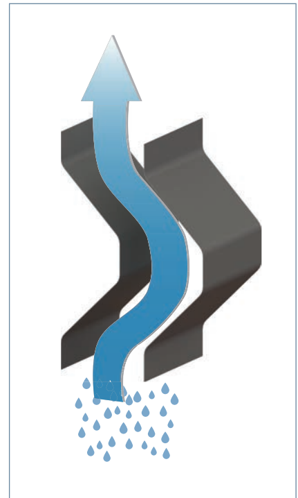
Vertical flow at the RV200 type profile
