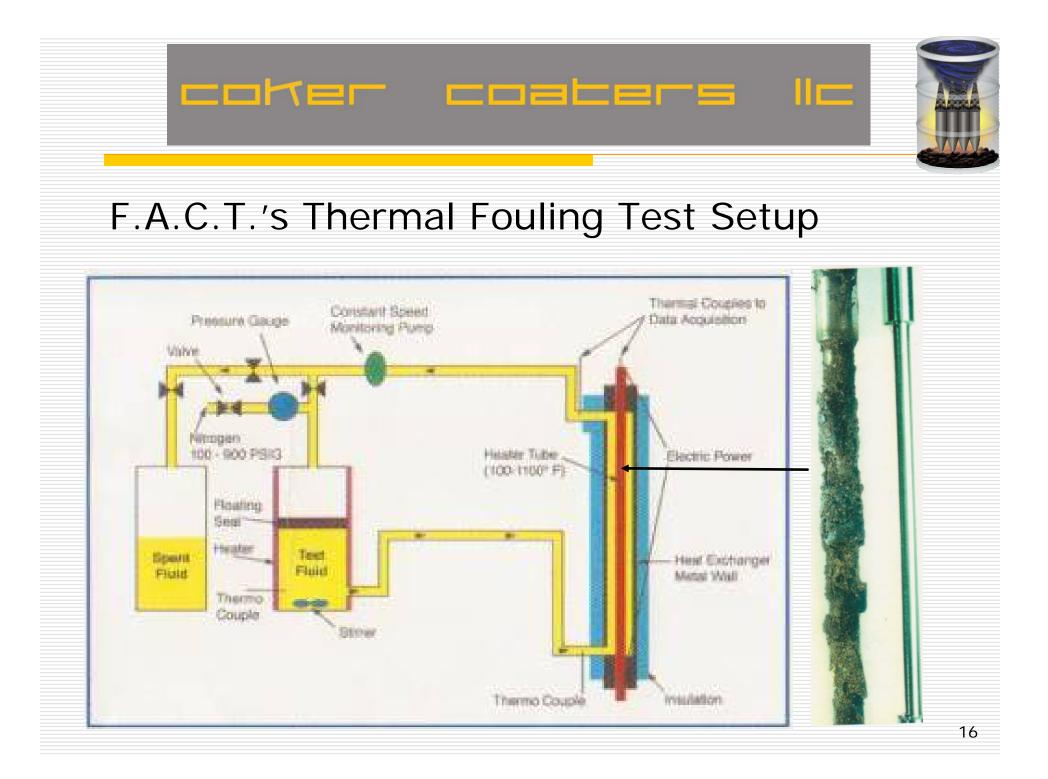
First, F.A.C.T. determines optimum fouling temperature of a given crude on an uncoated heat exchanger (heat exchanger simulates delayed coker furnace conditions).
