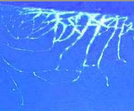
Cracks clearly visible after fluorescent spray
