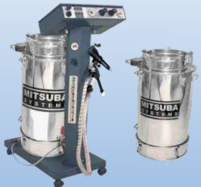
Pneumatic Hopper Mounted Siever ( 0 to 60 kgs/hr )
