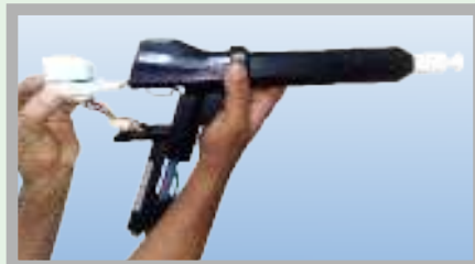
replace the power cartridge
