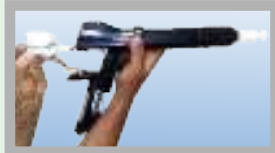
replace the power cartridge
