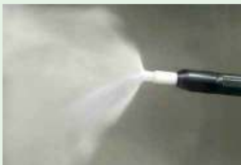
NORMAL GUN WITHOUT SIEVING - MILD STREAKING
