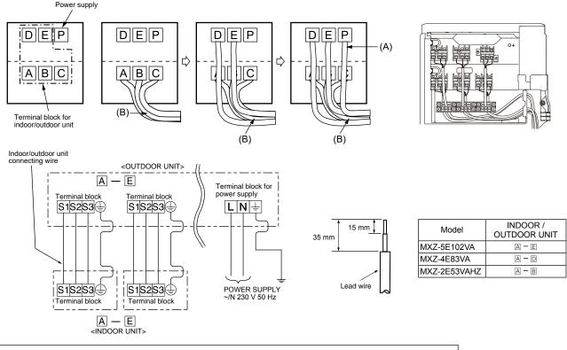
Be sure to attach each screw to its correspondent terminal when securing the cord and/or the wire to the terminal block.
