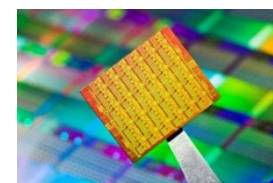
Single-chip Cloud Computer (SCC) of Intel contains 48 P54C Pentium cores (Intel ,2009)
