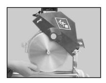
(E) Install Diamond Blade onto Blade Shaft
