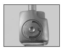
(A) Check that the Cooling Flow Adjusting Valve is FULL open
