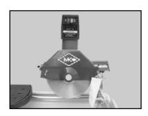
(I) Tighten the Blade Guard Retaining Wingnut
