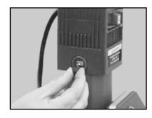
(B) Remove the Motor Brush Housing Cover
