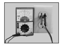
(D) Check power source voltage is 120v - if not 120v, move to another circuit
