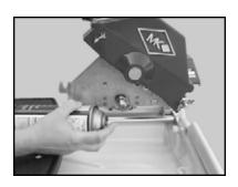
(C) Lubricate the Motor Shaft
