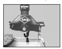
(A) Loosen the Blade Guard Retaining Wingnut
