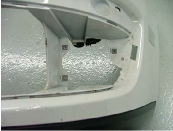
Speed clip inserts installed.
