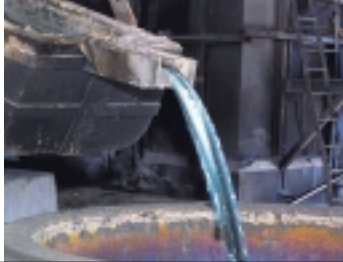
Pouring of tin metal for refining
