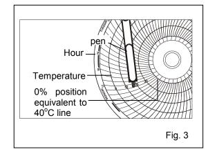
**NOTE:** There is a difference of approximately 2 mm between the red pen and blue pen during recording. The time difference between the red pen and blue pen changes according to their position on the scale. It is roughly two hours for 0% position of chart center and roughly one hour for 100% position (when the recording chart speed is set to seven days).
