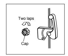
A door may not open in the above method when there are frost and ice in the air intake port. In that case, open a cap, and investigate the matter whether there is no frost inside the air intake port. Remove frost inside the air intake port in "the air intake port cleaning stick" of the accessories when there is frost. Clean a air intake port every month even when there is no frost inside the air intake port. Refer to page 24.
