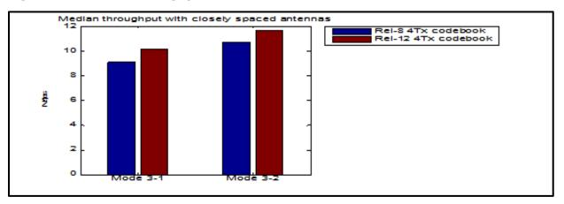
Figure 47: Median Throughput of Feedback Mode 3-2 and New Codebook.<sup>118</sup>
