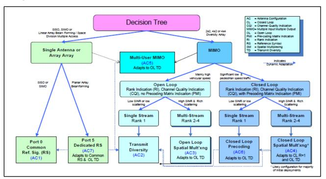
Figure 44: Decision Tree for Different Antenna Schemes<sup>115</sup>
