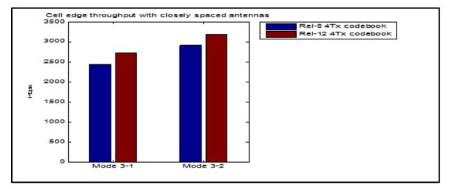
Figure 48: Cell-Edge Throughput of Feedback Mode 3-2 and New Codebook<sup>119</sup>
