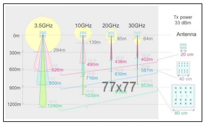
Figure 15: Range Relative to Number of Antenna Elements<sup>37</sup>
