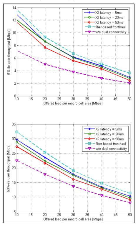
Figure 76: Dual Connectivity User Throughput<sup>168</sup>
