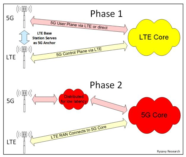
Figure 17: Two-Phase Approach to 5G Deployment
