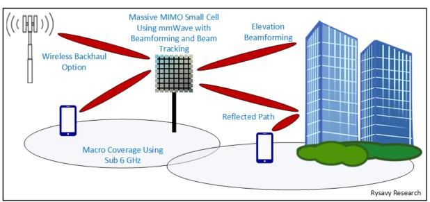
Figure 16: 5G Likely Architecture for Low Band/High Band Integration.
