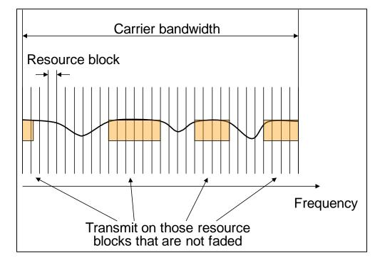
Figure 43: Frequency-Domain Scheduling in LTE<sup>113</sup>
