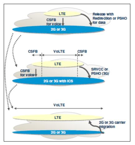
Figure 63: Evolution of Voice in an LTE Network<sup>150</sup>
