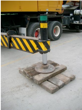
Figure 3 - Crane outrigger foot on timbers
