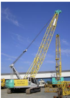
Figure 6 – Lattice boom crawler crane
