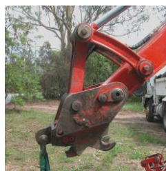
Figure 7 and Figure 8 - Lifting attachment with a closed eye on excavator
