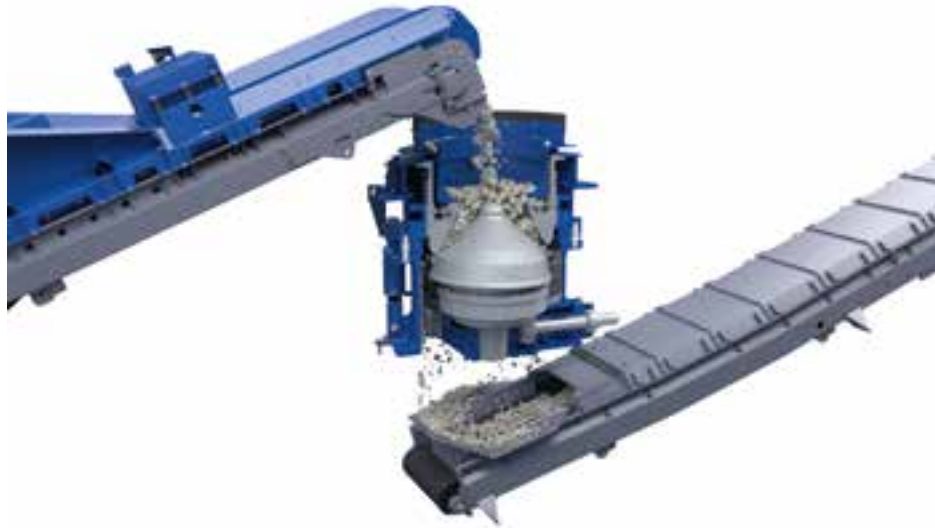
Crushing mechanism of cone crusher
