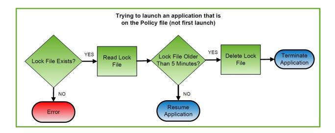
Figure 14: Launching a permitted application (not first launch)
