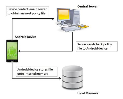
Figure 5: Main components of the intercommunication structure
