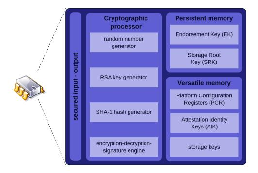
Figure 1: Trusted Platform Module security features [4]
