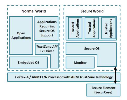
Figure 2: ARM TrustZone security architecture [7]
