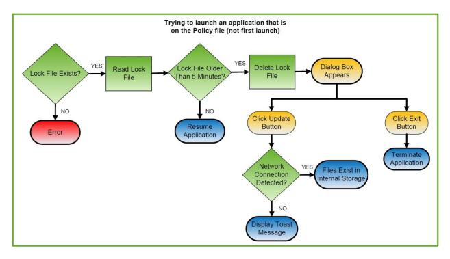
Figure 17: Launching a permitted application (not first launch) - renovated scenario
