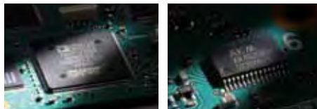
-DSP unit- ADSP-21369 Internal clock speed: 333MHz 32-bit floating point DSP Max. performance: 2000MFLOPS
