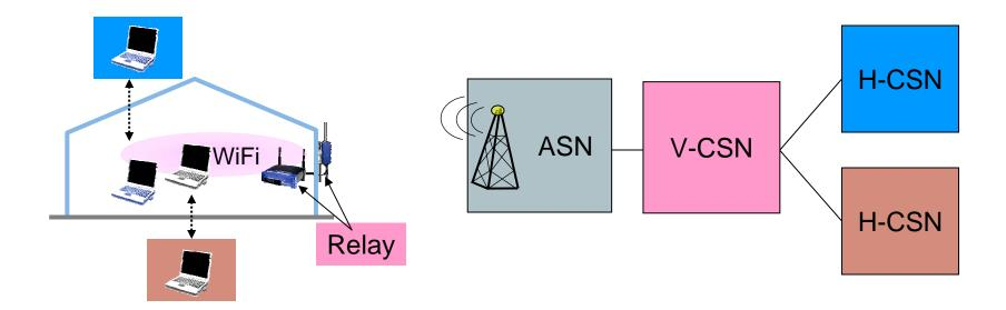
WiMAX-WiFi relays are providing deep-indoor coverage as well as connectivity in hot-spots and moving environments (e.g. trains)
