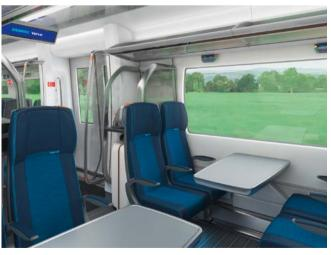
The seating has been designed taking ergonomics as well as additional space and passenger comfort for intercity travel into account. The standard seats have a slim visual aesthetic that lends a contemporary design appearance to the Standard Class saloon and creates a feeling of spaciousness in the vehicle.
