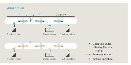
As a hybrid vehicle, Desiro Verve can also operate without catenary, which increases its efficiency and enables an optimised succession of trains on partly electrified lines – for minimised fuel consumption and reduced lifecycle costs.
