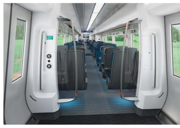
All seats and tables are cantilevered from the body side to provide completely unobstructed floor space.
