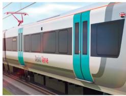
Desiro Verve can even be equipped with single-leaf end doors or double-leaf plug sliding doors at 1/3 – 1/3 position.
