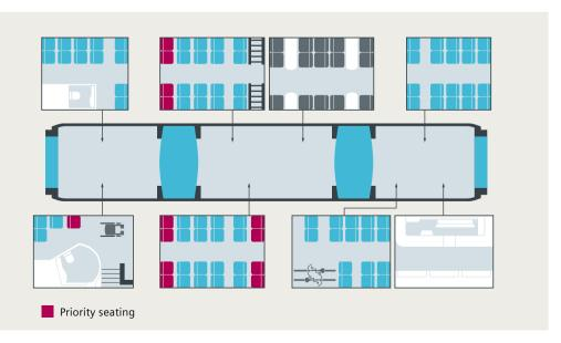
Thanks to the "empty car-body" concept, the entire layout is fully flexible. The interior and all door configurations can be converted again and again with minimal effort.
