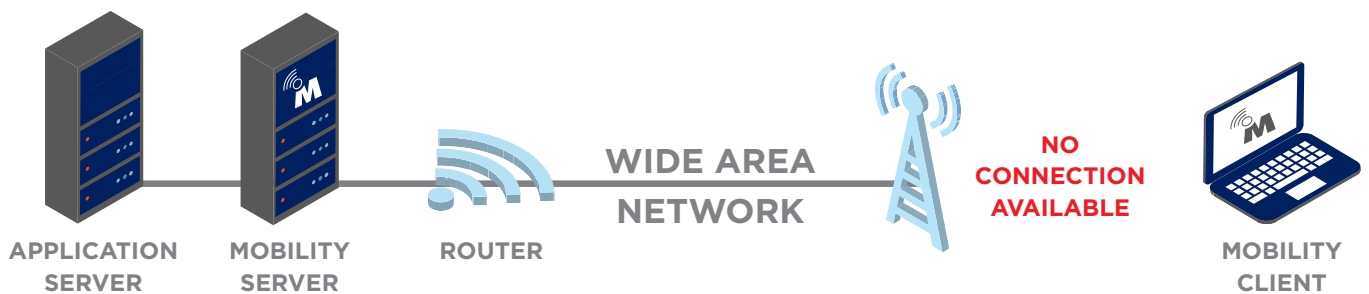
Mobility preserves the VPN tunnel, applications and data even when the client is unreachable.
