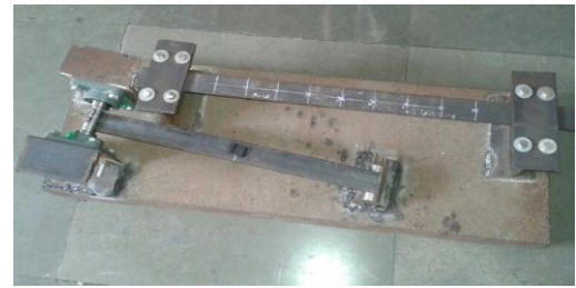
Fig 12 Combined Setup for Simply Supported & Fixed Beam
