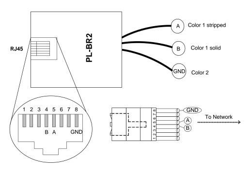
The PL-BR2 is a simple tool that converts the NET A, B and GND wires from an RS485 system into a female RJ45 port. The alignment of the wires in the RJ45 port corresponds to the official Modbus protocol. All ProLon devices also follow this protocol for their RJ45 ports. The main purpose of this device is to allow you to use a simple, unmodified Ethernet cable (CAT5) to connect two RS485 ProLon nodes together.
