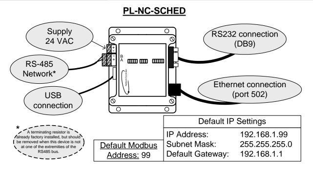
The PL-NC-SCHED has two main functions. The first is to act as an Ethernet to RS485 converter, used to convert the Modbus TCP/IP protocol into Modbus RTU serial protocol, allowing a user to view his whole ProLon zoning system from the internet. Its second function is to provide scheduling information to any device on the ProLon zoning system.
