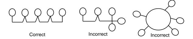
To connect VC1000 devices in a bus topology, the <u>NET A</u> port of one VC1000 device must be connected to the <u>NET A</u> port of the VC1000 devices directly preceding it and following it in the bus. The same must then be done with the <u>NET B</u> wires. If the NET wires are mistakenly inverted, LED#5 on the VC1000 device will turn ON and it will not be able to communicate. However this will not affect the other VC1000s on the network.
