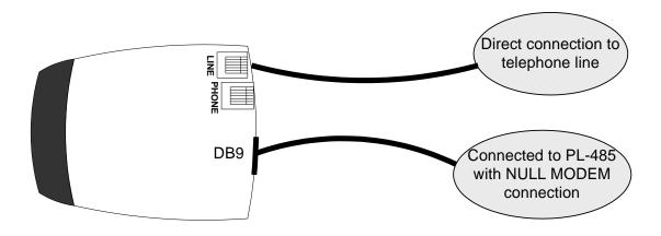
To connect to a VC1000 network from a computer over a phone line, your computer must first be equipped with a modem. If you are using ProLon Focus, Focus automatically configures the modem for you. Otherwise, you must determine the proper configuration for your software.
