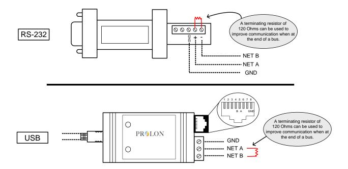
The PL-485-USB is an RS-485 bidirectional converter. It is used to allow a computer or modem to communicate properly with the VC1000 system.
