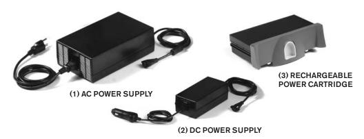
The ECLIPSE charges the optional Power Cartridge when external power (AC or DC) is present and when the Power Cartridge temperature is below a safe charging temperature. When external power is disconnected, the system will automatically switch over to the Power Cartridge, if installed. When external power is restored (by plugging into AC or DC outlets) the system will accept power from the external source and replenish the Power Cartridge while operating, if adequate power is available.
