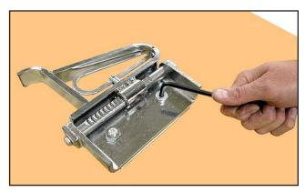
Figure 8 - Removing the SHCS
