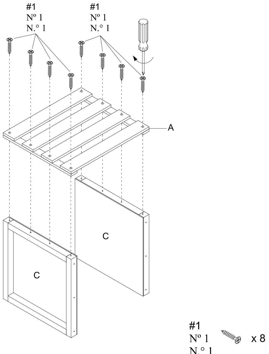
**Step 2.** Attach long panel (part B) to short panels (part C) using screws (part #1) and phillips head screwdriver. Repeat for remaining long panel.
