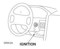
Once the lower dash panel has been removed, locate the ignition harness at the back of the key cylinder. This is usually a group of thicker wires. With the ignition harness exposed, use your digital multi-meter to find your power and ignition wires.
