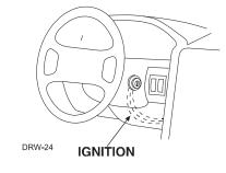
Now that the accessories have been located, find the wire suspected to be the starter wire according to the web information on your vehicle. Place the red lead of your meter on the wire. With the key in the off position the meter should read 0.00 volts and will stay at 0.00 volts in all key positions except the crank position. In the crank position your meter should read between 10.00 volts and 13.00 volts, and will drop back to 0.00 volts when the starter disengages.
