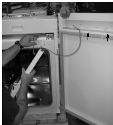
Figure 6-14. Move Wires To Right Side
