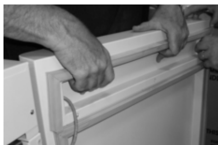
Figure 6-15. Install Top Pan & Gasket
