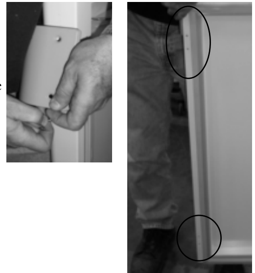
Figure 6-13. Remove Hinges, Display Frame
