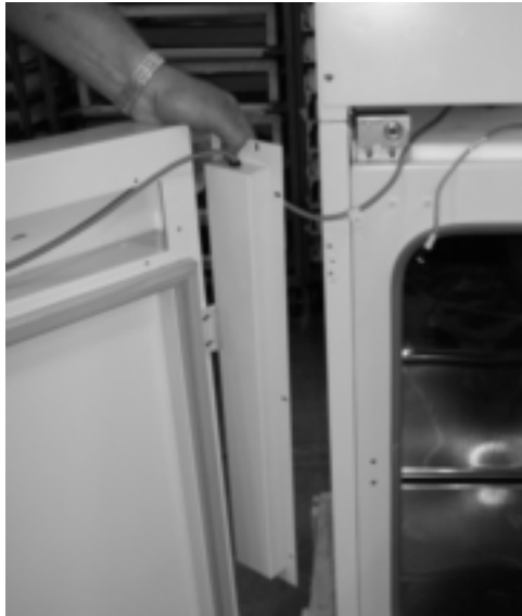
Figure 6-11. Set Door and Pan Aside
