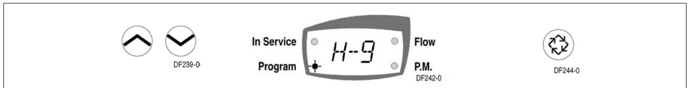
Figure 9: Feed Water Hardness
