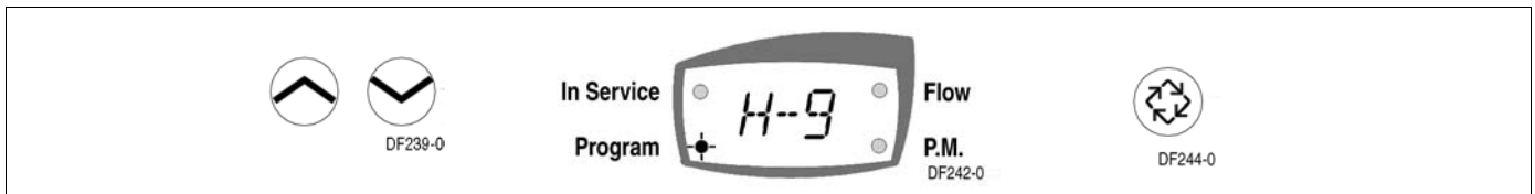
Figure 5: Feed Water Hardness
