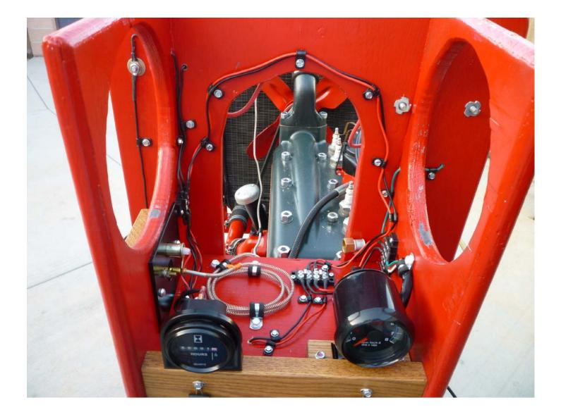
Wiring inside the control panel to the ignition and all the gauges. The hour meter is on the left; the tachometer is on the right. The backside of the gauge on the left side panel is the water temperature gauge. The EGT gauge is directly below it.
