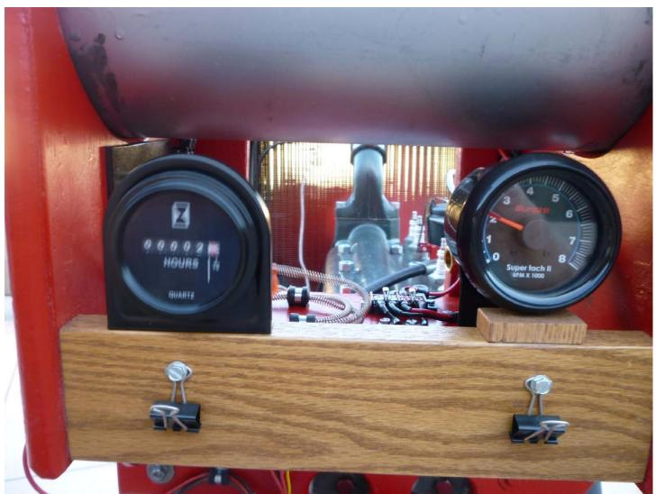
The running time meter and tachometer are mounted to the backside of the control board. Below are two clips to retain notes about the engine status. The gas tank is directly above.
