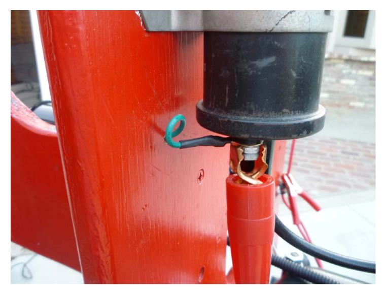
The input signal for the tachometer is taken off the low side of the coil. The gauge is set for a four-cylinder engine. The clip lead is the connection to the distributor cable.
