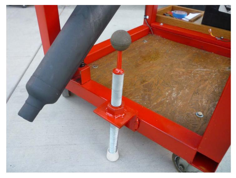
A parking brake is installed to keep the engine stand from taking off down the road.
