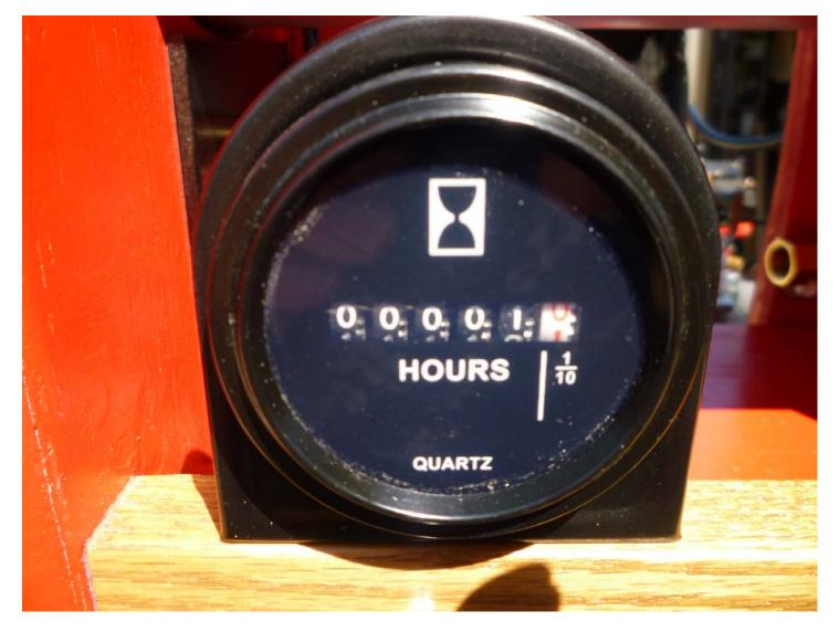
A running time hour meter records the total time the engine has been run in the test stand. The reading is cumulative. When a new engine is installed in the test stand a notation has to be made of the current reading on the gauge before starting the test.
