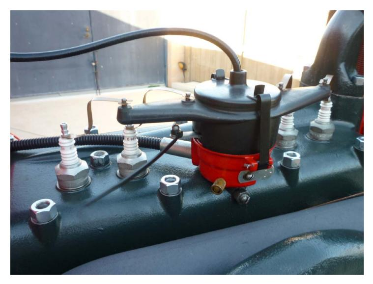
The distributor has a tie wrap attached to the spark advance lever for convenience of setting the advance. When timing a test engine the distributor upper section has to be temporarily mounted and the spark advance lever pulled toward the manifolds until it is up against the stop. This is the fully retarded position and duplicates the position it would be in if it were connected to the advance lever in a Model A.
