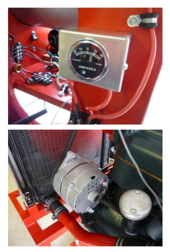
An ammeter was installed in the electrical system. It will show any discharge from a connected electrical load when running the engine with the idler pulley instead of an alternator or generator (top photo).
