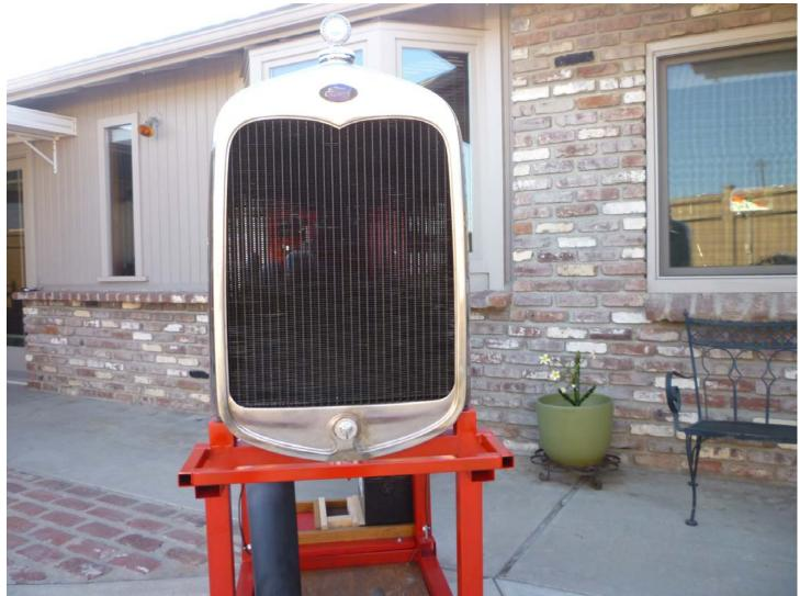
A 1930 radiator shell and a radiator cap has been installed.
