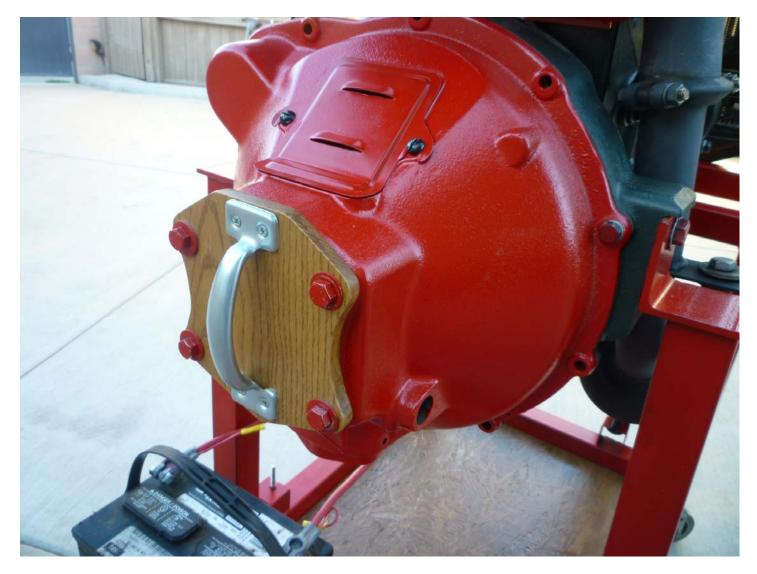
A dummy bell housing is installed as a safety feature to enclose the flywheel. The handle it to facilitate moving the test stand around.
