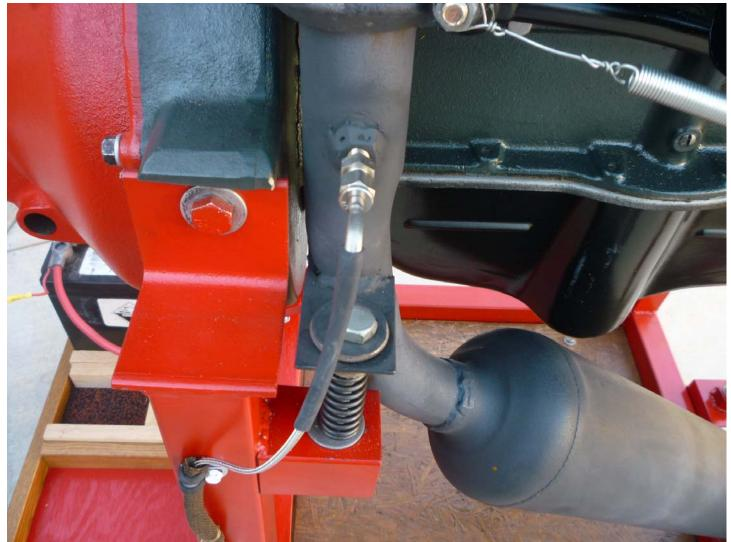
The modified Model A muffler is attached to the frame on spring loads and is left in place when the engine is removed from the test stand. The probe for the EGT gauge is located just below the muffler clamp. A threaded boss is welded to the header pipe for the probe to insert. When an engine is removed the probe stays in place with the muffler and is disconnected at the gauge.
