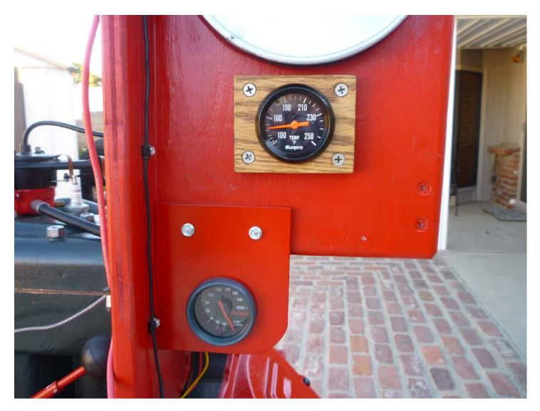
The water temperature gauge is mounted to the left side of the control board just below the fuel tank. The gauge contains a backlight connected to 12-volt power for nighttime operation.
