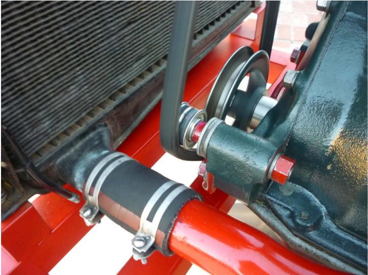
An idler pulley supported by two bearings is mounted in place of a generator and takes up the slack of the fan belt.
