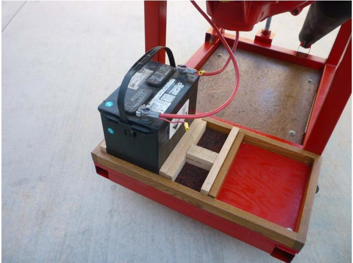
The engine test stand compartment will accept any size 12-volt battery. Blocks of wood are positioned to prevent the battery from walking around due to engine and stand vibration.
