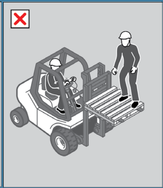
FIGURE 13 Using a forklift as a working platform or to gain extra height by standing on the tynes or a pallet is an unacceptable practice.
