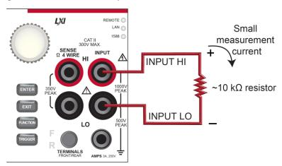
Figure 22: DMM7510 front-panel 2-wire resistance measurement
