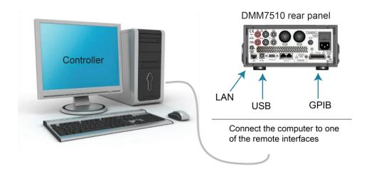
Figure 13: DMM7510 remote interface connections
