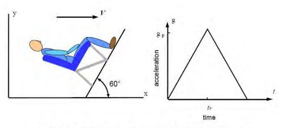
FIGURE 1-1. FOURTEEN-g DYNAMIC SLED TEST CONDITIONS
