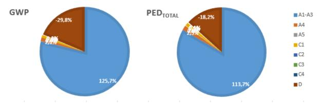
In relation to reinforcement steel, the importance of each module for the total life cycle result is illustrated in Figure 34, for the two categories indicated above.
