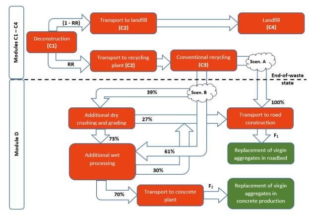
Figure 18. End-of-life stages concrete [46]
