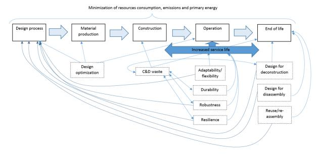
Figure 5. Links between aspects of structural design over the life cycle
