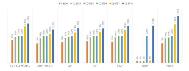
Figure 14. Environmental impact indicators for different concrete grades
