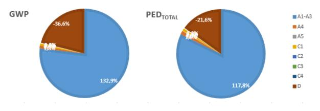
**Figure 34.** Importance of each module in LCA of steel reinforcement (base scenario)
