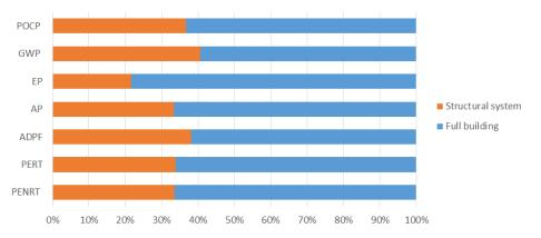
Figure 58. Weight of the structural system in relation to the whole building
