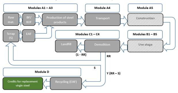
Figure 32. Model for LCA of steel products
