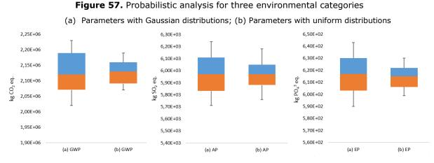
In this case, the two probabilistic analysis lead to very similar results in terms of the median values. The scatter of values is higher for the Gaussian distribution than the uniform distribution. However, it is observed that the scatter of results in Figure 57 would increase if uncertainty was considered also in Modules A1 - A3.
