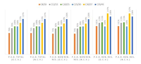
Figure 15. Primary energy indicators for different concrete grades
