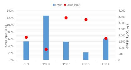
Figure 30. GWP for 1000 kg of steel section from GaBi and EPDs from Table 26.
