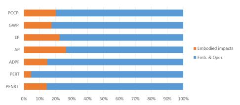
Figure 50. Weight of embodied impacts in the LCA of the building
