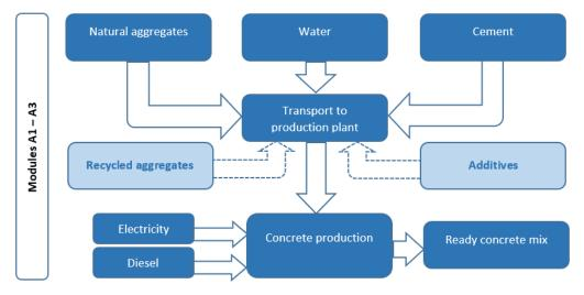
Figure 13. Production of concrete (Modules A1 – A3)
