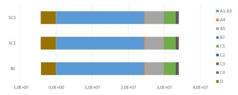
Likewise, given the importance of Modules A1-A3, the variation of the final aggregated results, for each scenario, is almost negligible, as observed from the above graphs.
