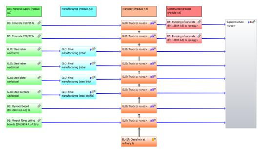
Figure 10. Processes included in the plan of the superstructure
