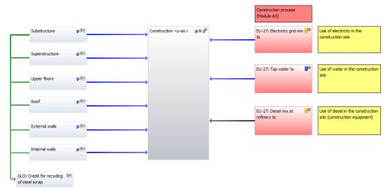
The substructure includes the preparatory works that are needed in the terrain for the construction of the building, the foundations and all auxiliary materials such as waterproofing membranes. All vertical load-bearing elements, such as columns and walls,
