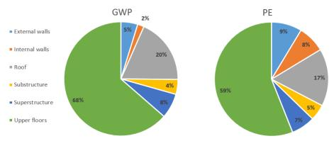
Figure 53. Contribution of building components in Modules A1-A3
