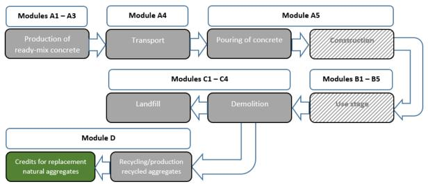
Figure 19. System boundary for LCA of concrete
