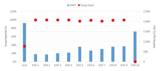
Figure 29. GWP for 1000 kg of steel rebar from GaBi and EPDs from Table 25.
